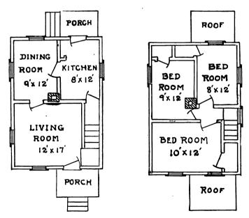
Fig. 43.—FIRST AND SECOND FLOOR PLANS OF DETACHED FRAME HOUSES FOR MINERS IN ANTHRACITE REGION.
